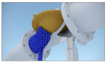
is released from the control chamber by an automatic or manual release device. The water supply pressure in the inlet chamber forces the diaphragm off the seat, allowing water to flow into the system and the alarm devices.
