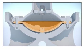
minimising the pressure loss through the valve. Model VD is specifically designed for harsh industrial environments such as onshore and offshore installations. It is suitable for use with sea water, foam concentrate or water foam solution. SA Fire deluge valves, Model VD, are **UL/cUL Listed**.
