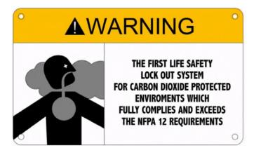
To avoid such situations in  $CO_2$  systems, NFPA 12 has included in its 2008 edition the introduction of lock off units to prevent accidental Carbon Dioxide discharge into the protected space. To avoid such situations in Inert Gas systems, the introduction of a shut off unit in the actuating circuit prevents accidental discharge into the protected
