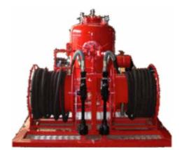
The fixed units can be equipped with selector valves for multiple protection with or without a 100% back up package.
