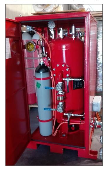
mass stream and is directed towards the burning surface of a protected target. Upon discharge on the fires, the particles penetrate and surround the fire atmosphere which is causing the combustion reaction. The dry chemical particles, in contact with the fuel and the strong heat, interact with free radicals in place of the Oxygen resulting in the combustion chain being inhibited and therefore suppressing the fire.
