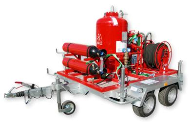
Each trolley is provided with a self-supporting frame designed according to the weight and speed with which the equipment is to be pulled. The wheels can be provided with road-type tyres that allow good manoeuvrability also on bumpy sections.
